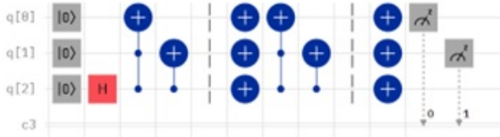
FIGURE 2 – Complete quantum circuit for the quantum walk in a cycle of 4 nodes.
