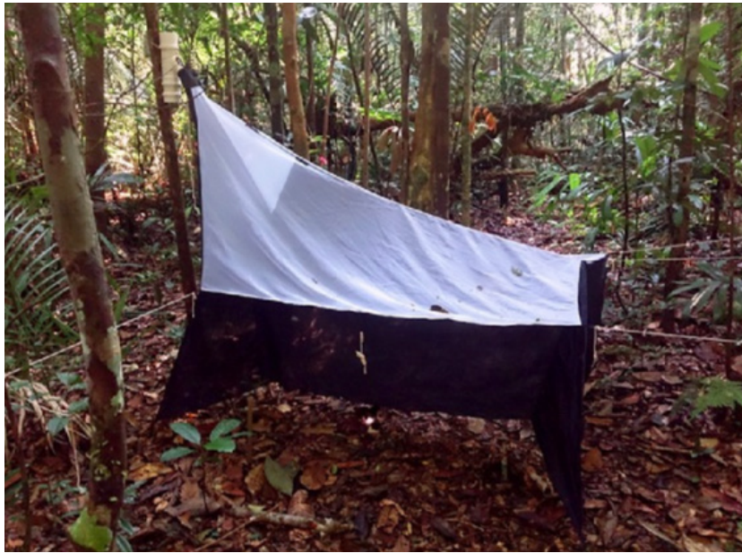
Fig 1. Malaise trap mounted perpendicular to a trail in Reserva Ducke (Image: Samuel S. Azevedo).
